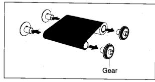
Pull out the four gears from the used film cores.
